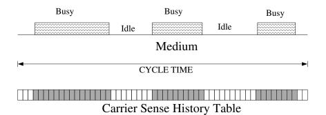
Fig. 3. Nodes use CSMA to monitor the medium and mark their current Carrier Sense History Table according to the sensed medium busy and idle times.
