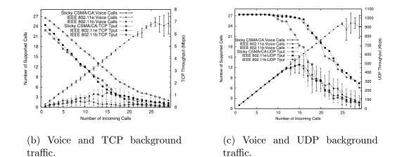
Fig. 14. Sticky CSMA/CA call carrying capacity for the irregular grid topology. All figures show 95% confidence intervals for the average number of supported calls.
