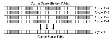
Fig. 4. At the beginning of each cycle, nodes derive their Carrier Sense Table as a summary of their Carrier Sense History Tables. The Carrier Sense Table helps to identify periodic real-time flows.
