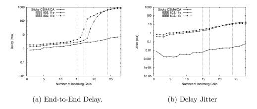
Fig. 17. Average end-to-end delay and delay jitter for voice calls over the over the irregular grid topology.
