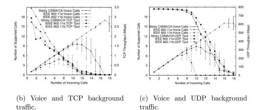
Fig. 11. Sticky CSMA/CA call carrying capacity for the line topology. All figures show 95% confidence intervals for the average number of supported calls.
