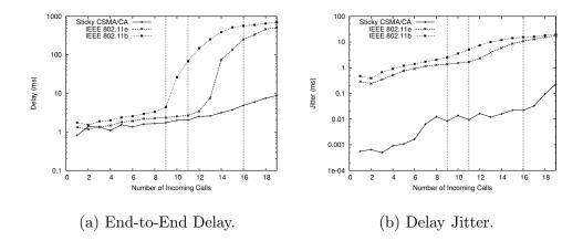
Fig. 15. Average end-to-end delay and delay jitter for voice calls over the line topology.
