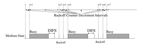
Fig. 6. Variable time-intervals between two consecutive backoff counter decrements at an IEEE 802.11 node.
