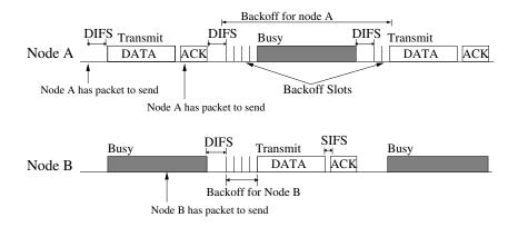
Fig. 1. CSMA/CA: Backoff mechanism
