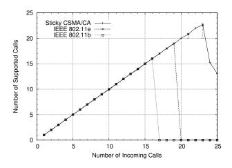
Fig. 7. The total number of voice calls supported as a function of the incoming calls for a two node network, with nodes 150m apart.
