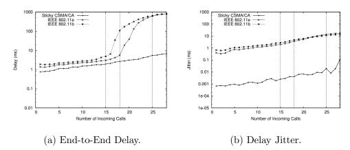
Fig. 16. Average end-to-end delay and delay jitter for voice calls over the regular grid topology.
