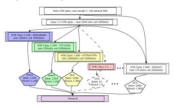
Figure 7: Traffic shaping design for Kwaabana using the Traffic Control subsystem of the Linux Kernel.
