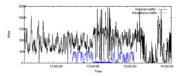
Figure 10: Plot of traffic passing through the gateway illustrating Kwaabana file synchronization and all other Internet traffic.
