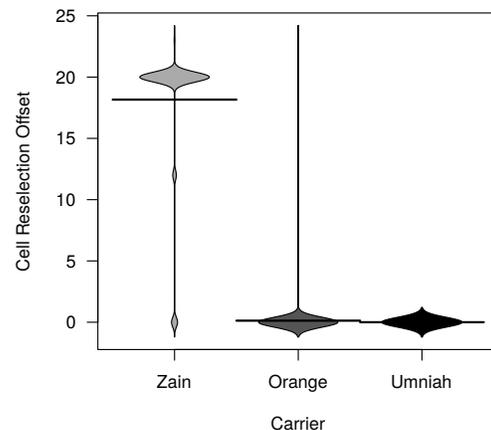
Figure 7: CRO artificially increases the calculated signal strength when the phone determines which cell to use.
