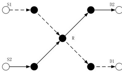
Figure 1: Intra-node interference at fixed wireless router  $R$ .
